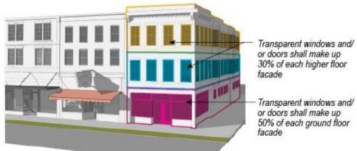
Figure 14 – Transparency Standards Example in Downtown District Overlay. Source 2021 Gallup Land Development Standards
